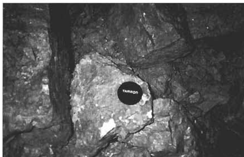
Fig. 4 - Limestone blocks in breakdown pile, Kozja jama v Pogorelem hribu. Note "weathered" surface of blocks. Blocks show continuing post-fall disintegration. Lens cap 55mm.
